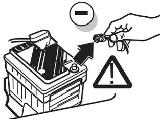
Note: It may be necessary to check if this vehicle has a stored radio code before disconnecting the battery!
